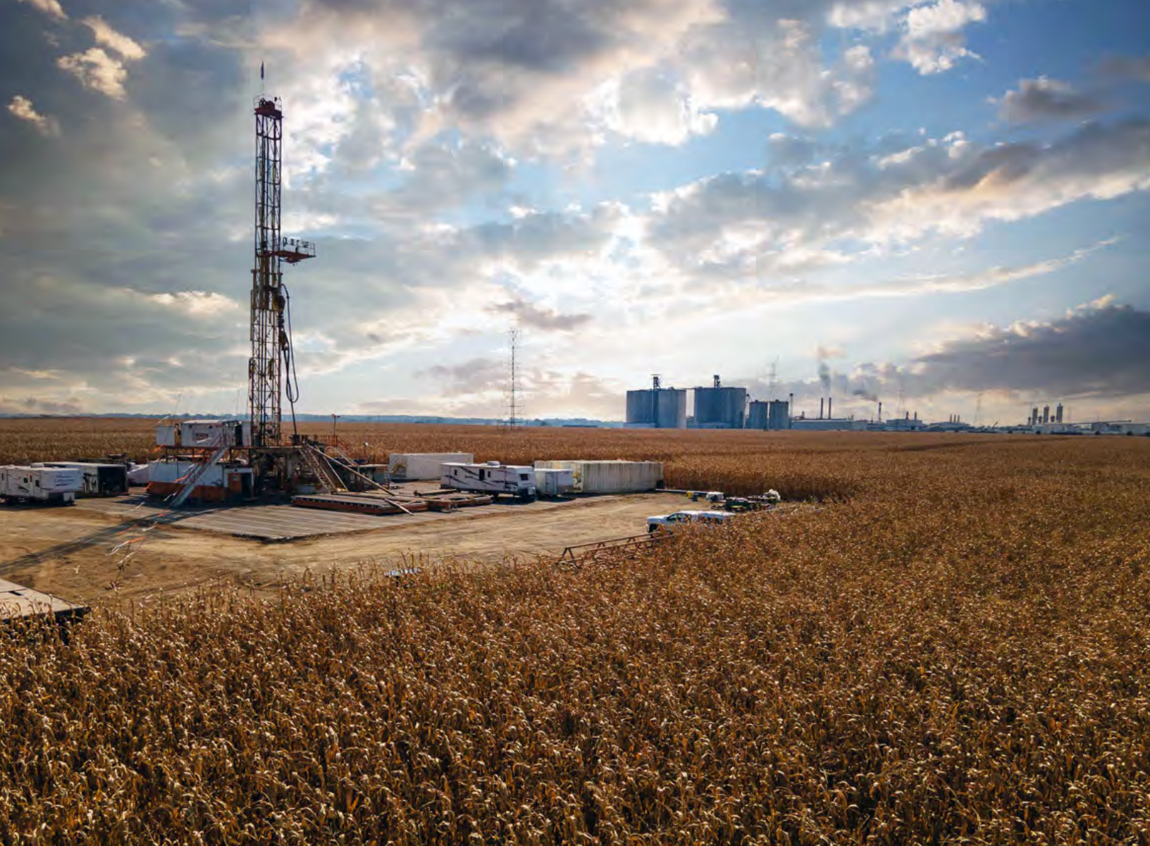
CCS FRONTIER: While Strategic Biofuels may become the first renewable diesel producer to capture and sequester CO 2 , the U.S. ethanol industry is aggressively pursuing CCS through pipeline aggregation and independent projects. Marquis Energy, the sixth ethanol producer in North America, has commissioned a 5,000-foot sequestration test well (shown here) at the site of its bio-industrial complex in Hennepin, Illinois.
