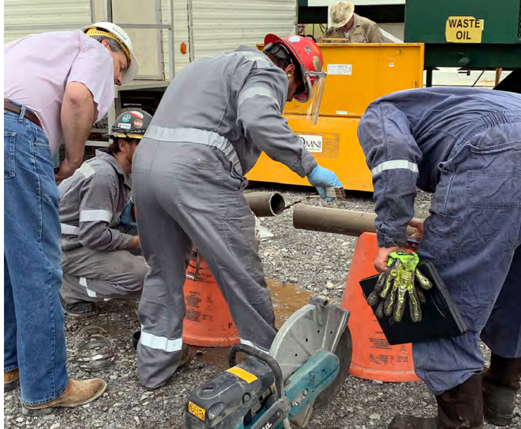
PIECE BY PIECE: Multiple 30-foot core sections were collected using the stratigraphic test well. To verify the presence of adequate upper and lower containment and injection intervals, each 30-foot section was cut into three equal sections for analysis.
